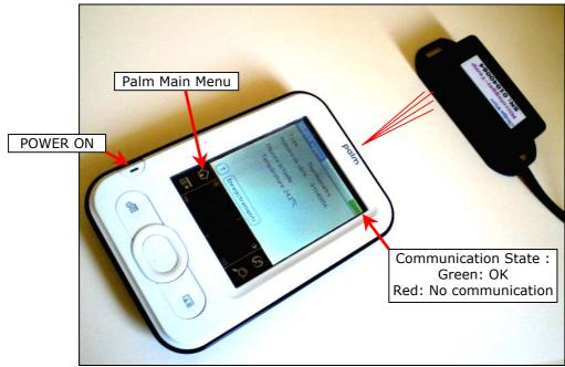
Example of IR communication using Palm Zire 22. Communication between a logger and a PDA
